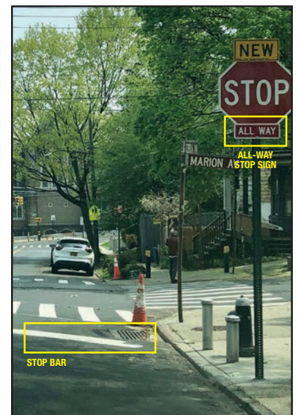
Figure 35. An example of an all-way stop-controlled intersection.
