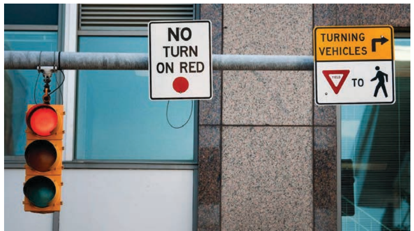
Figure 43. An example of a no-turn-on-red sign.
