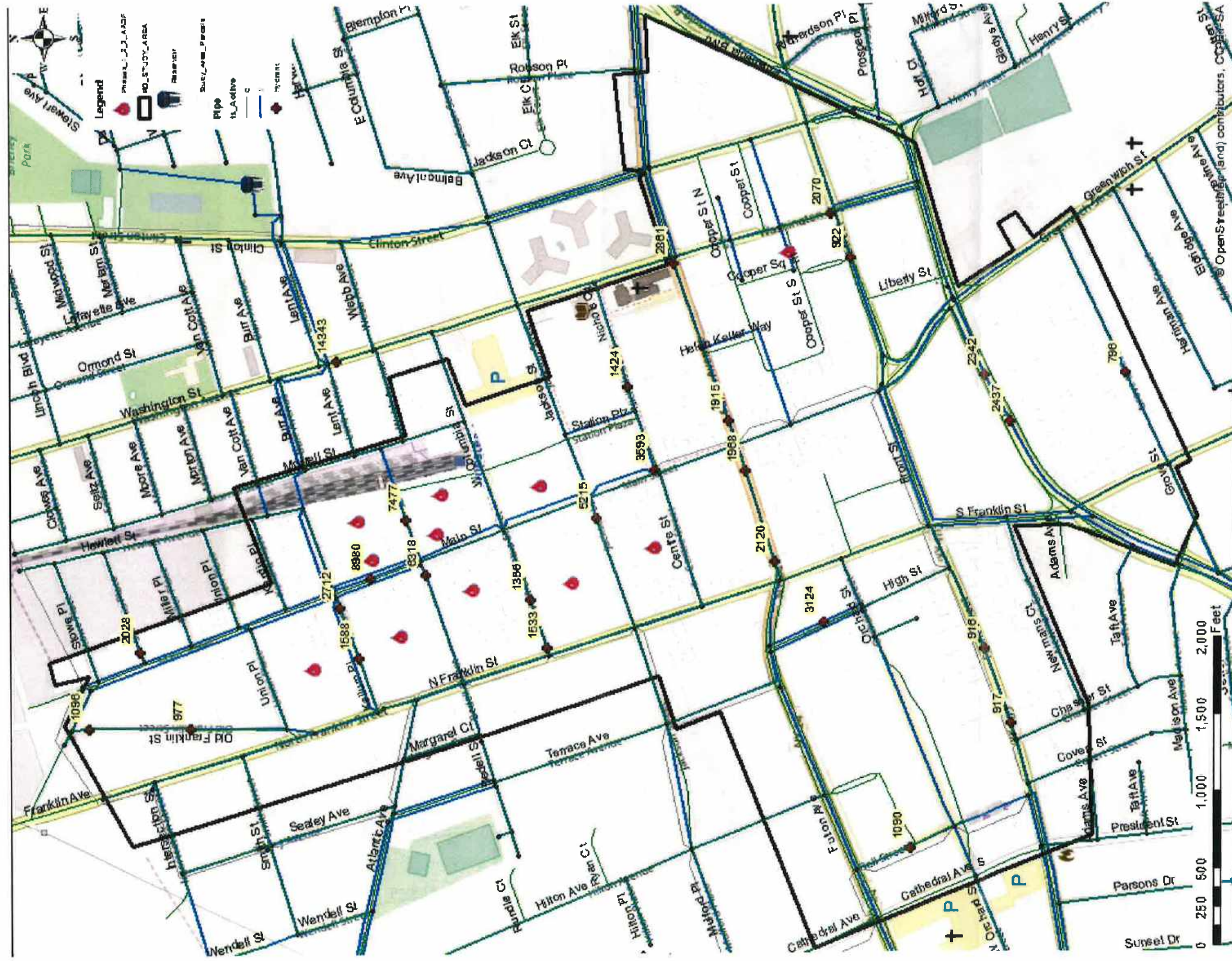
Figure No. 11 – Scenario 2, Available Fire Flow with Phase 1 & 2 Improvements plus 2300 LF 12 inch on Main; Kellum to Center Street
