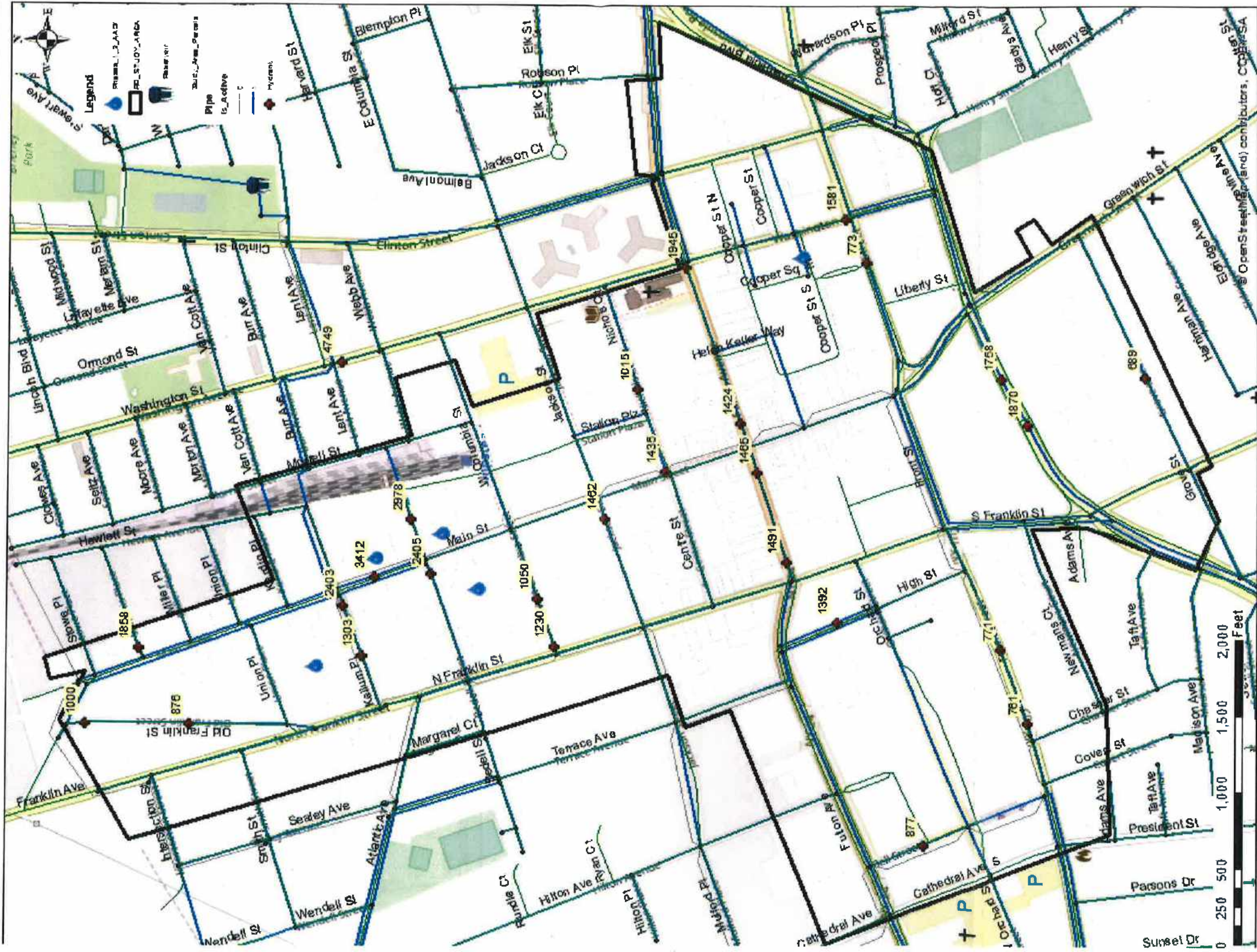
Figure No. 8 – Scenario 1, Available Fire Flow with Existing Pipes PLUS 1910 LF of 24 Inch Main and Phase 1 & 2 Demands
