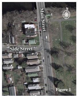
Side Street and 25 seconds of green time for Main Street every one minute. This signal is a "fixed time" signal, meaning it gives that 25 seconds of "green time" to each approach regardless of whether traffic is present or not.
